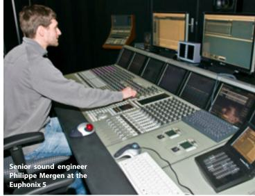
the PA system and simultaneously to 96 kHz capable Euphonix A/D converters, which are installed beneath the stage. The signals are then sent via fiber optics to the recording studio. Inside the studio an output at the mixing desk again creates a digital splitter, allowing the signals to be forwarded to a broadcast truck.
